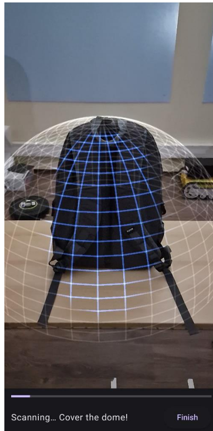
3. Figure: During scanning, the Luma AI app artificially illuminates the environment on the device's display. It does not turn on the flash of the device.
