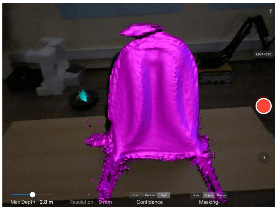
2. Figure: Scanning process with 3D Scanner App. The LIDAR sensor detects the scanned object correctly even in poor lighting conditions.
